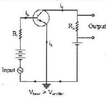
This has been shown a n-p-n transistor. Therefore, base-emitter are forward biased and Input signal is connected between base and emitter.
